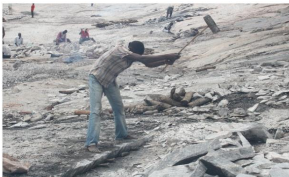
Plate I: Quarry worker using hammer to break the rock fragments as required by the end users
