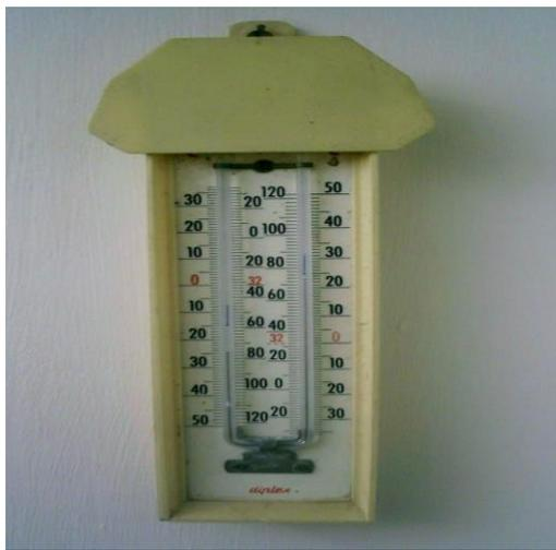
Figure 2: A Typical Outdoor Minima-Maxima Thermometer
