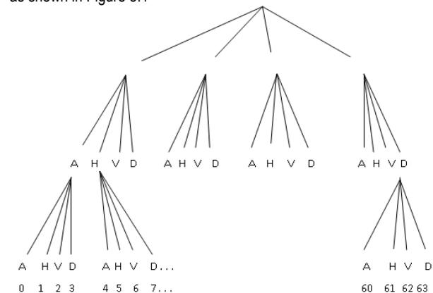
Figure 3.1: Wavelet Packets Decomposition
