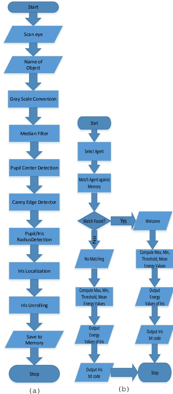
Figure 3.2: Iris acquisition and authentication enhancement flow diagram
