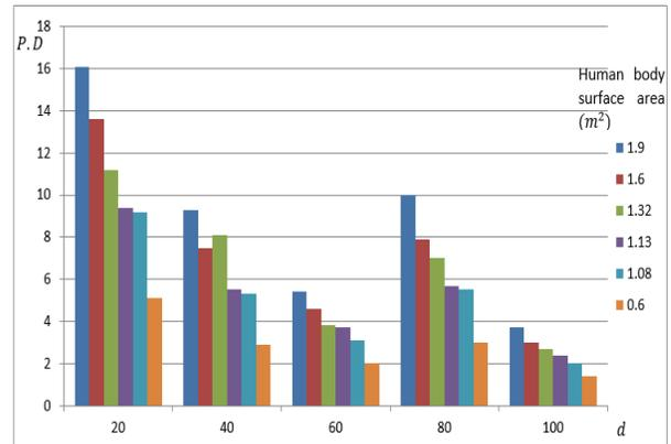
**Figure 2** Average Power density versus distance from the 42 selected BTS stations
