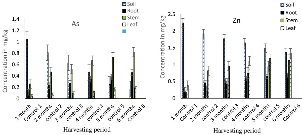
**Figure 4.0:** The concentrations (mg/kg) of As and Zn from exposed soil and plant part and control soil and plant part on each harvesting period
