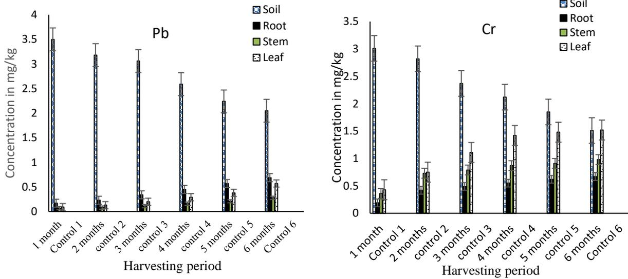
**Figure 3.0:** The concentrations (mg/kg) of Pb and Cr from exposed soil and plant part and control soil and plant part at each harvesting period
