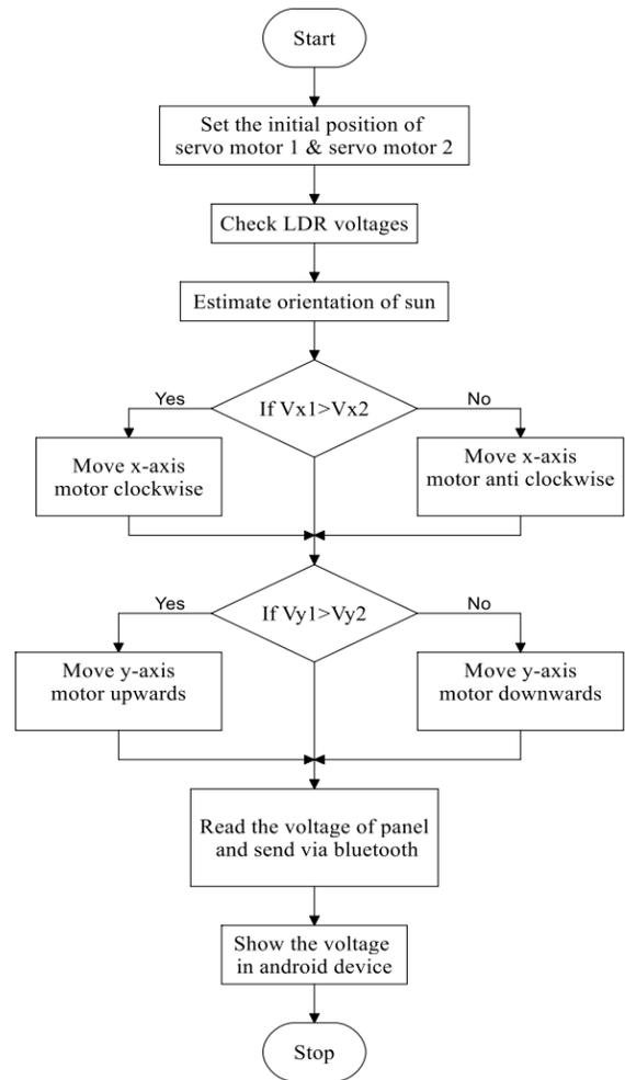
Fig. 2. Block Diagram of Process
