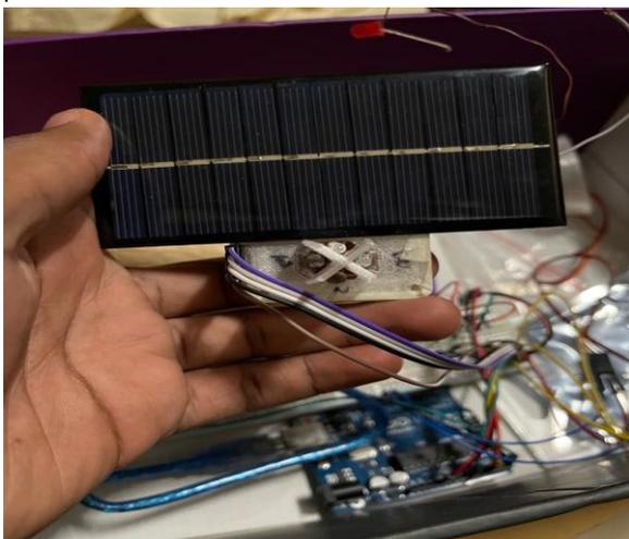
Fig. 5. LDR sensor position
