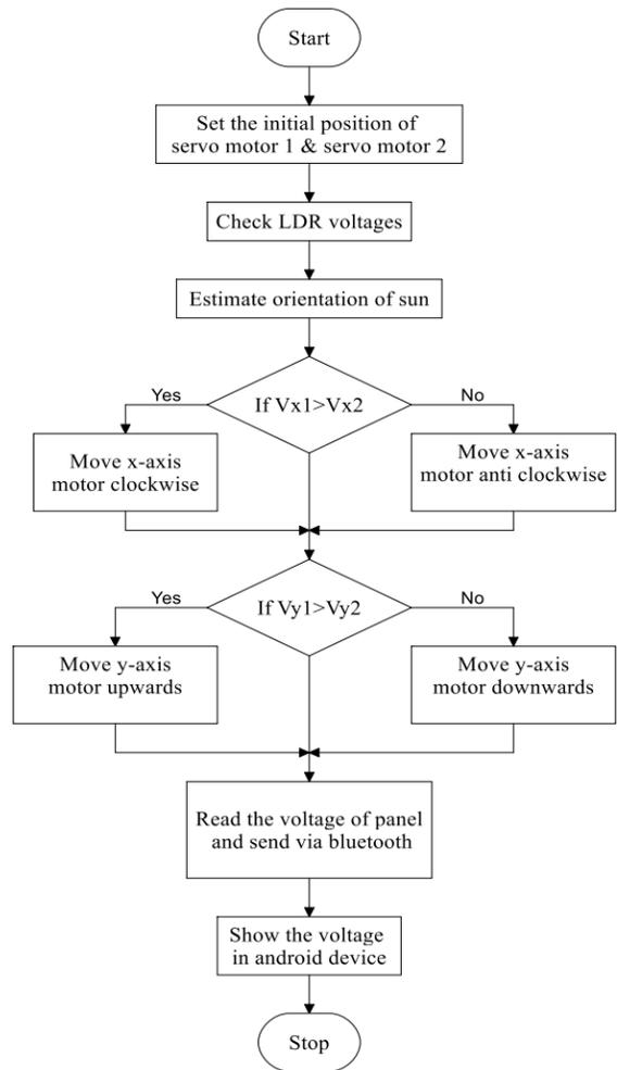
Fig. 2. Block Diagram of Process
