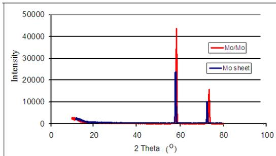
Figure 2. XRD of molybdenum sheet and sputtered molybdenum
