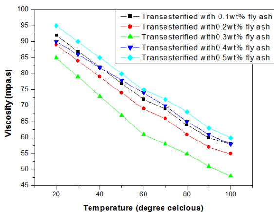
Figure 3: Viscosity of Trans-esterified Neem Oil with 0.1wt%, 0.2wt%, 0.3wt%, 0.4wt%, and 0.5wt% fly ash with Temperature
