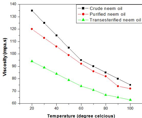
Figure 2: Graph of Viscosity of crude neem oil, purified neem oil and trans-esterified neem oil
