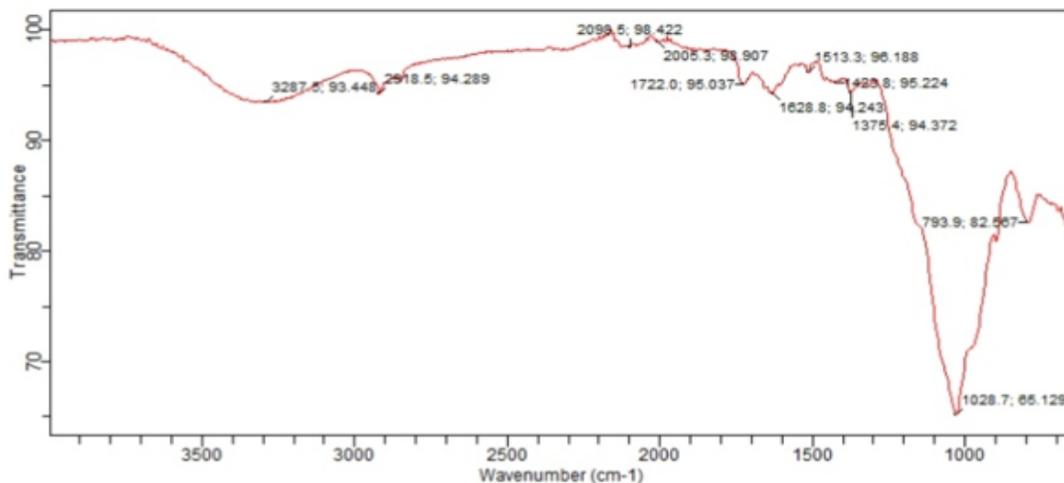
**Figure 1:** ATR- Fourier transform infrared spectroscopy of untreated Maize Fiber
