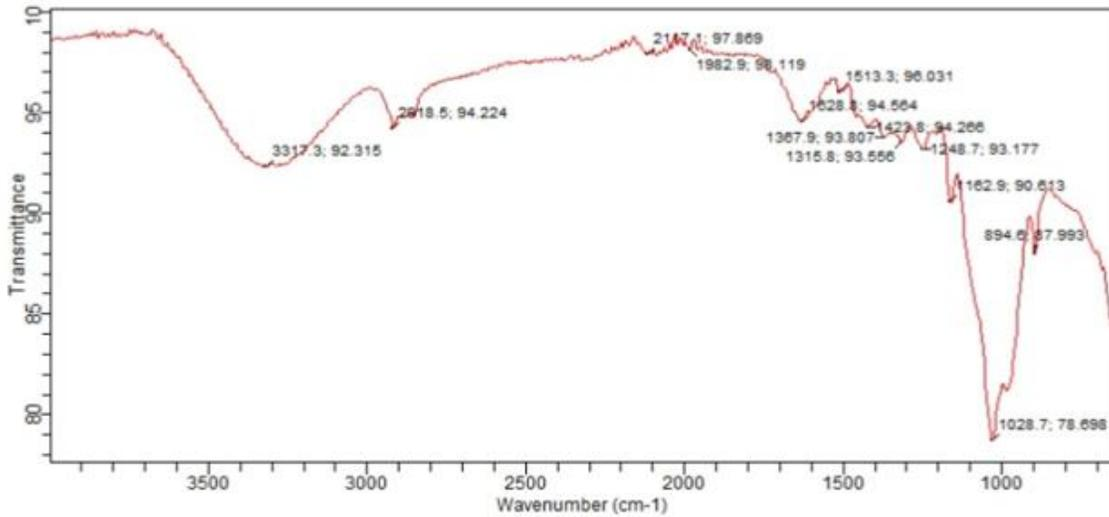
Figure 3: ATR- Fourier transform infrared spectroscopy of Treated Maize Fiber
