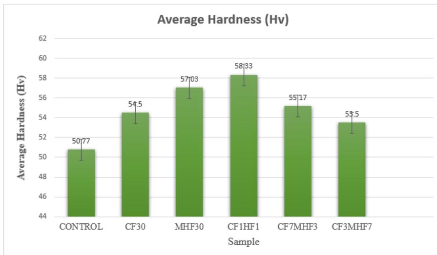
**Figure 9:** Hardness Test of prepared CF/MH hybrid Composites
