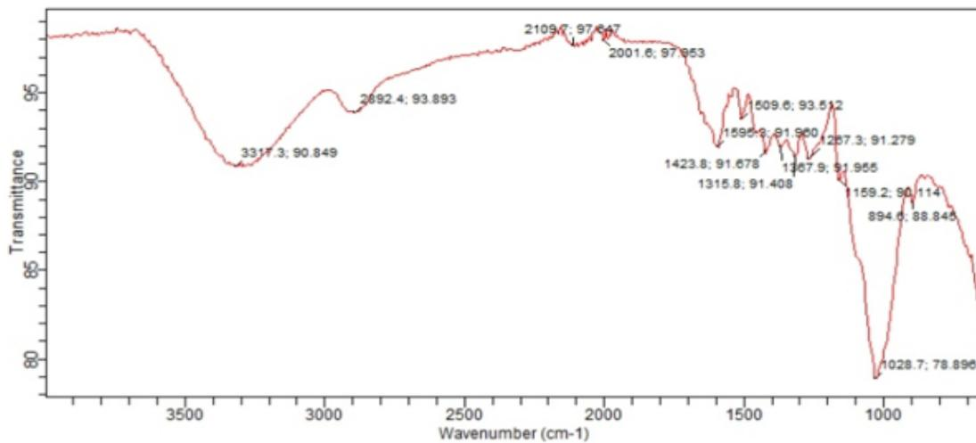
Figure 4: ATR- Fourier transform infrared spectroscopy of Treated Coir Fiber
