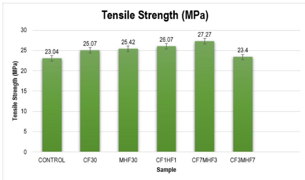
**Figure 6:** Tensile Strength of Prepared CF/MH hybrid Composites
