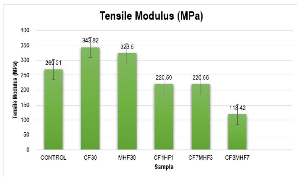
**Figure 7:** Tensile Modulus of Prepared CF/MH hybrid Composites
