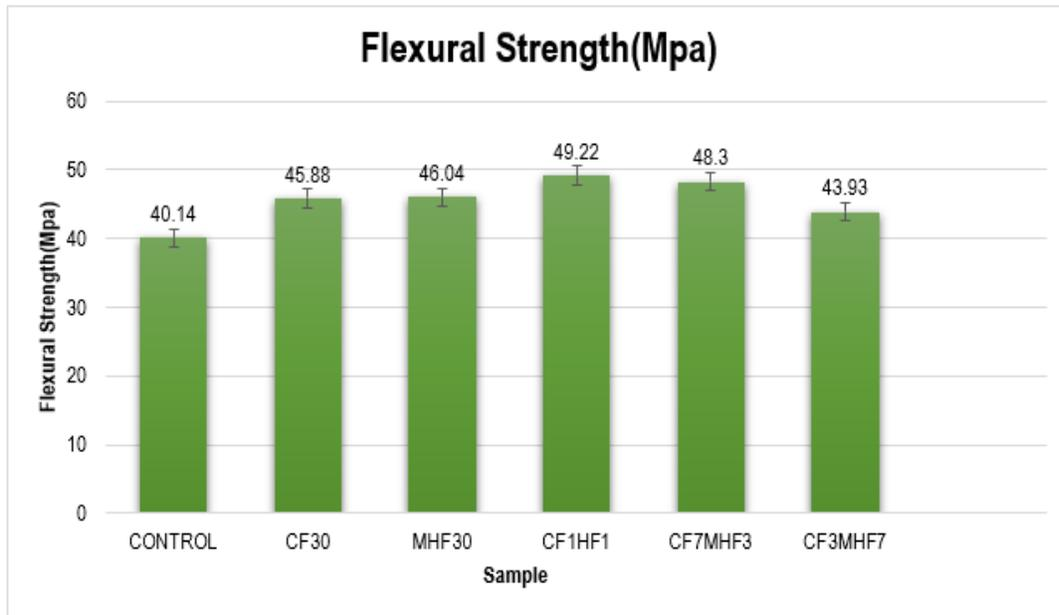
**Figure 11:** Flexural Strength of the CF/MH hybrid Composites
