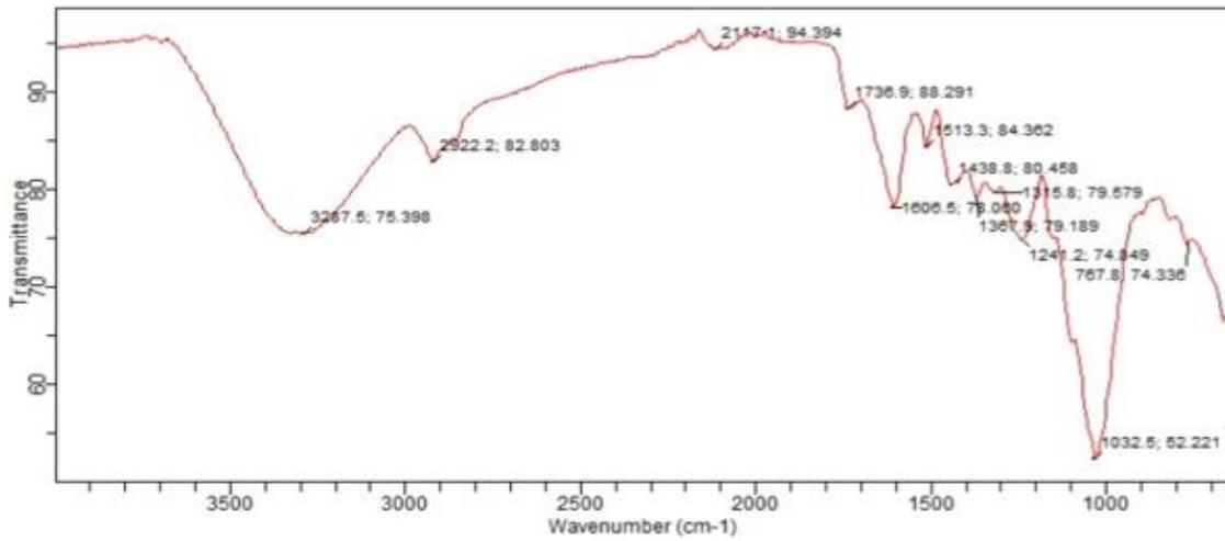
Figure 2: ATR- Fourier transform infrared spectroscopy of untreated Coir Fiber
