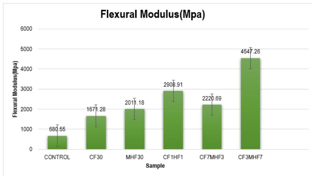
Figure 10: Flexural Modulus of the CF/MH hybrid Composites
