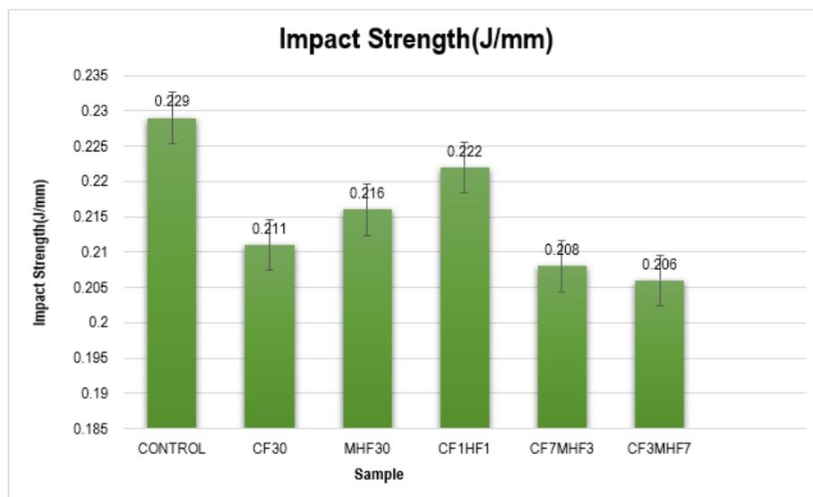
**Figure 8:** Impact Strength of prepared CF/MH hybrid Composites
