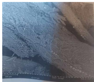
Figure 1: SEM Micrograph of uncarbonized Barassu aethiopium seed (magnification = 1000)
