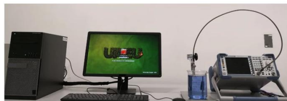
Figure 2. Complex Permittivity measurement using open-ended coaxial probe.
