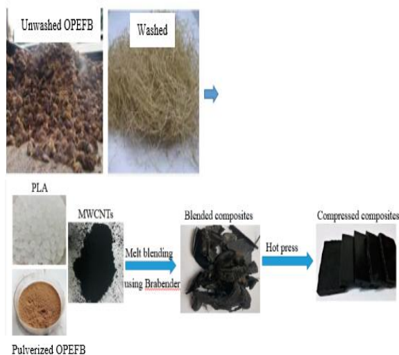
Figure 1. Fabrication of OPEFB/PLA/MWCNTs composites
